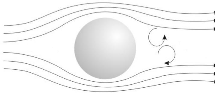
$$\underbrace{F_D}_{\text{dependent}} = f \left( \underbrace{V, \rho, \mu, D}_{\text{independent variables}} \right)$$
